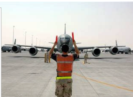
Maintaining KC-135s, turning fuel into freedom Senior Airman Mike McGovern marshalls a KC-135 Stratotanker to its parking spot at a deployed location in Southwest Asia while Tech. Sgt. Robert Wade and Senior Airman Neal Sicard stand by to place chocks around the tires of the aircraft. The Airmen are with the 340th Aircraft Maintenance Squadron. (U.S. Air Force photo/Staff Sgt. Jason Barebo)
